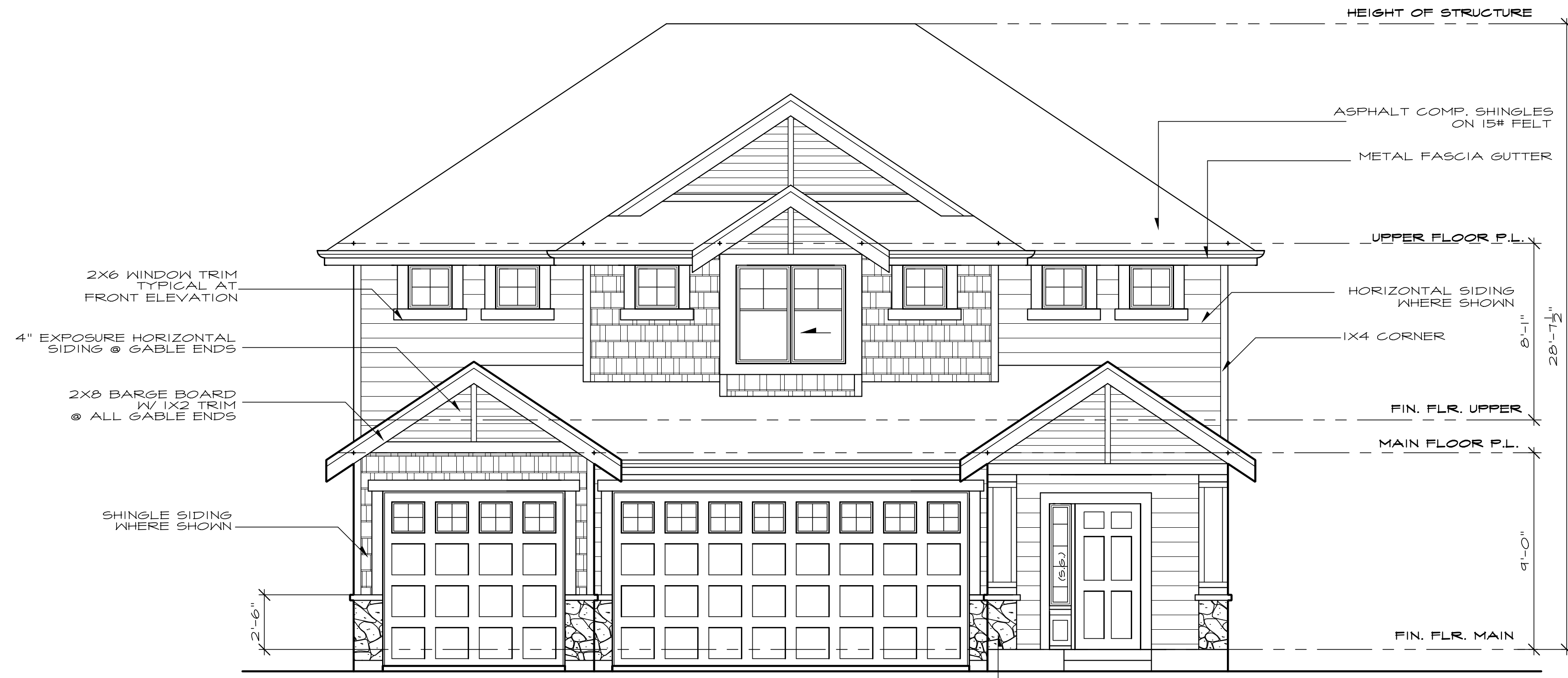
CULTURED STONE VENEER INSTALL PER MFD. SPECIFICATIONS TREATED PLYWOOD BEHIND ALL AREAS WITH STONE FRONT ELEVATION
